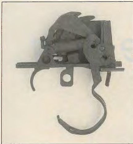
M14/M1A trigger assembly, (left) shown here with the hammer cocked and the trigger guard down for disassembly purposes, was lifted right out of the .30 M1 Garand. (right) M14/M1A trigger assembly with the hammer forward in the fired position.
